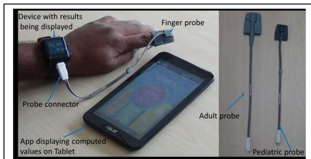
Figure 1. Wrist based wearable monitor along with the smart phone/tablet and custom probes
